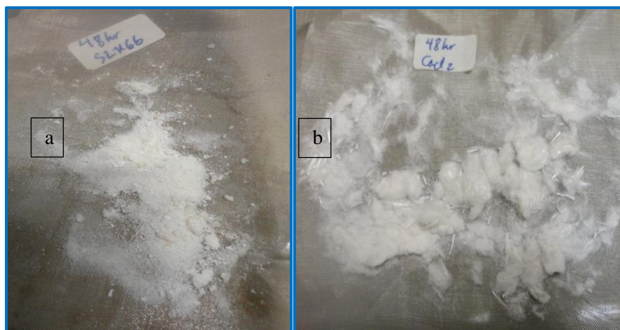
Figure 2: fiber in 10% mutual solvent + 20% CaCl 2 after drying in oven (right) and fiber in 20% CaCl 2 after drying in oven (left)
