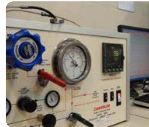
ULTRASONIC CEMENT ANALYZER (REAL-TIME MONITORING OF CEMENT COMPRESSIVE)
